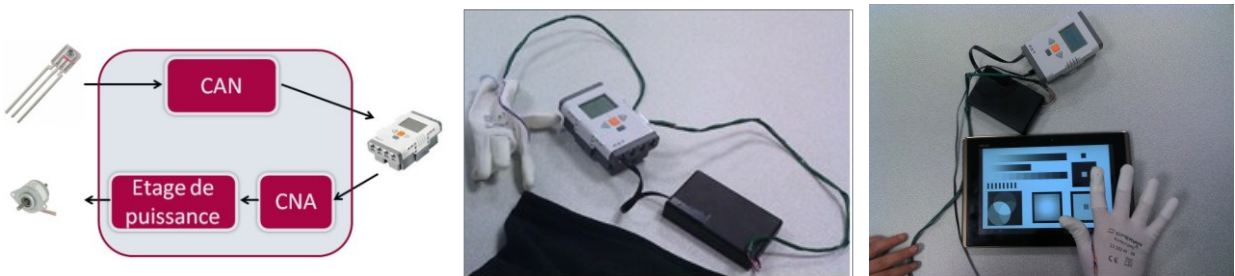
Fig. 4. (a) Framework Architecture; (b) Vibro-Tactile framework; (c) Framework with the Digital Tablet.
